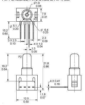
2 x 2 Termination (Style 2) Port Style A, Straight Pin 1 is notched, Pin 1 is shown at lower right corner. Pins 2, 3, 4 are clockwise.
