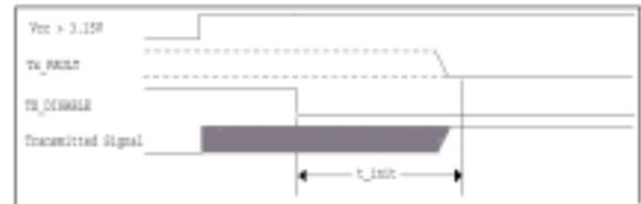
Power on initialization of GBIC, TX_DISABLE asserted
