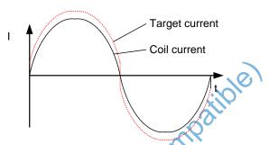
Coil current does not have optimum shape
