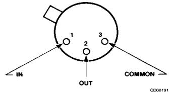
Lead 3 connected to case.
