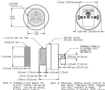
NOTE A: TERMINALS—0.32 BRASS TIN PLATED, TAPPED FOR #6-32 SCREW. TWO #6-32 NICKEL PLATED BRASS SCREWS INCLUBED. WILL ACCEPT 1/4\* QUICK CONNECT.
