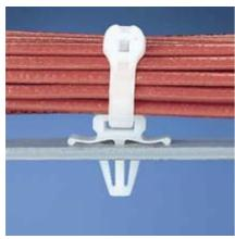
Push mounts require no adhesive backing or additional mounting hardware. They are inserted into pre-drilled holes. The winged base applies pressure on the panel wall to provide a more secure mount in high vibration applications. Can be used where only one side of panel is accessible.
