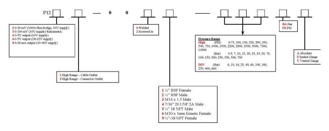
Example: P1283-0023-10KPSS = 4 to 20mA output, connector outlet, screwed in M14 male port, 10,000 psi sealed gauge
