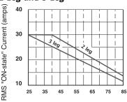
Ambient temperature (°C), measured 1 inch (25mm) below relay when mounted to DIN rail or a vertical, 1/8th inch thick aluminum panel surface. Airflow is unrestricted up and through the heat sink.
