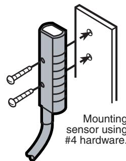
Mounting sensor using #4 hardware.
