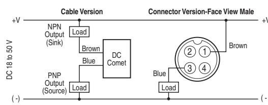
**CAUTION:** AC/DC connector version sensors use an AC-type connector. Use of DC power with AC-type connectors may not conform with established standards.
