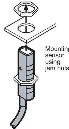
Mounting sensor using jam nuts.
