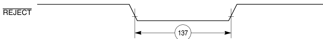
Figure 64. CAM Interface \overline{\text{REJECT}} Timing Diagram
