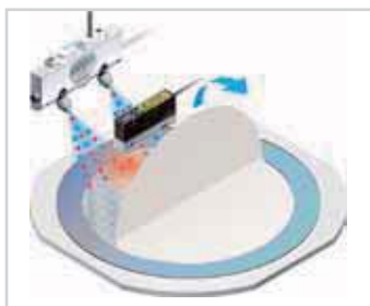
Measuring surface potential when removing BG sheets
