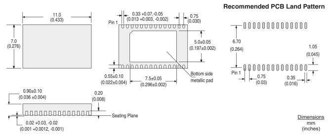
NOTE: Because the metallic pad on the bottom of the DFN package is connected to the substrate of the die, IXYS Integrated Circuits Division recommends that no printed circuit board traces cross this area to avoid potential shorting issues.
