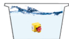
IP67: Submersion to one meter for 30 minutes.
