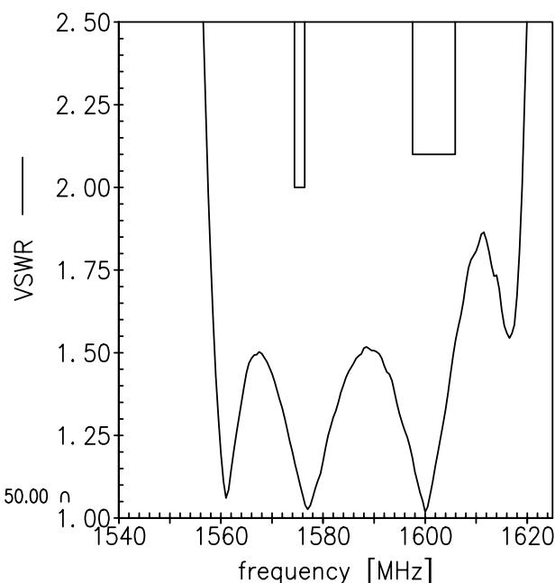
**SAW Components****B9482****SAW GPS + GLONASS Filter****1590.16 MHz****Data Sheet**
