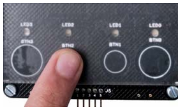
Figure 3-8. Broken Link in BTN2-LED2
