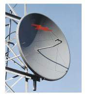
4.6 m | 15 ft Standard Parabolic, Low VSWR Unshielded Antenna, single-polarized, 7.125–8.500 GHz, CPR112G, gray antenna, with flash, standard pack—two-piece reflector
