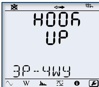
Hook up, voltage and current ratios and aggregation period can be configured from the front panel of the PEL 103.
