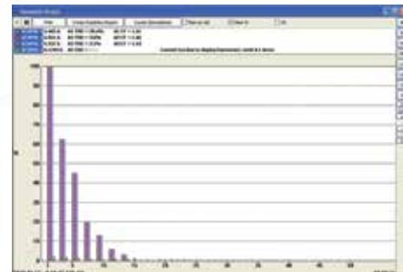
Display all harmonics from 1<sup>st</sup> to 50<sup>th</sup> in bargraph form for voltage, current and power.
