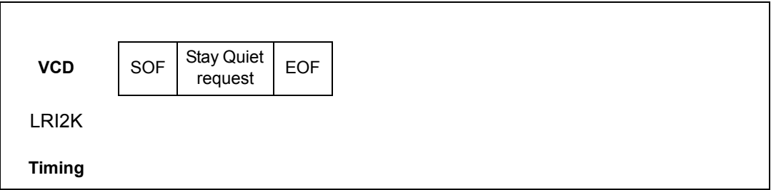
Figure 40. Stay Quiet frame exchange between VCD and LRI2K
