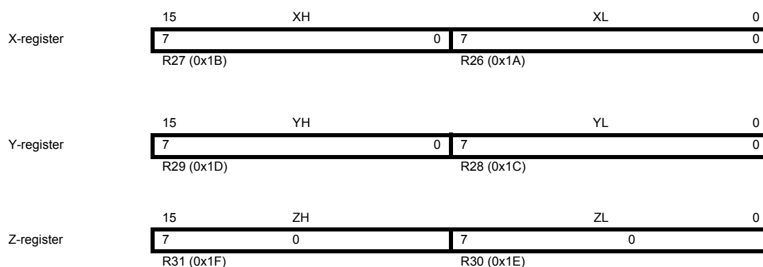
Figure 7-3. The X-, Y- and Z-Registers
