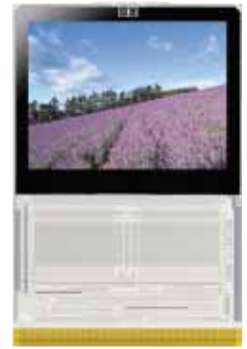
TFT color LCD module featuring LSI with DRAM frame memory integrated onto the glass substrate (prototype)
