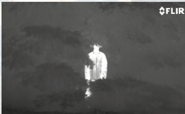
Thermal imaging: person hiding in bushes is clearly visible since thermal contrast is practically impossible to mask.
