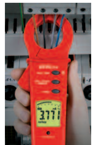
differential current measurement method
