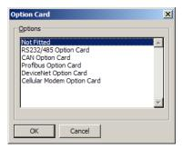
Selecting the appropriate card will add an icon to tree shown in the left-hand pane of the window. This icon will in turn contain icons for the additional port or ports that are made available by the card. The example below shows a Gateway with a serial expansion card installed...
