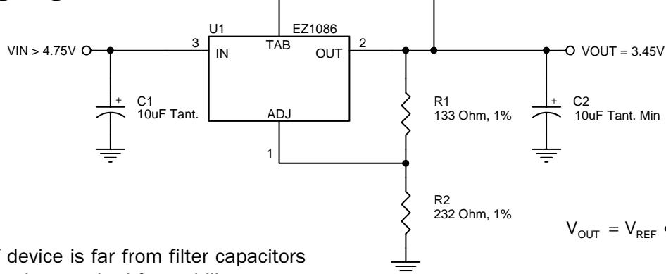
$$V_{OUT} = V_{REF} \cdot \left(1 + \frac{R2}{R1}\right) + I_{ADJ} \cdot R2$$
