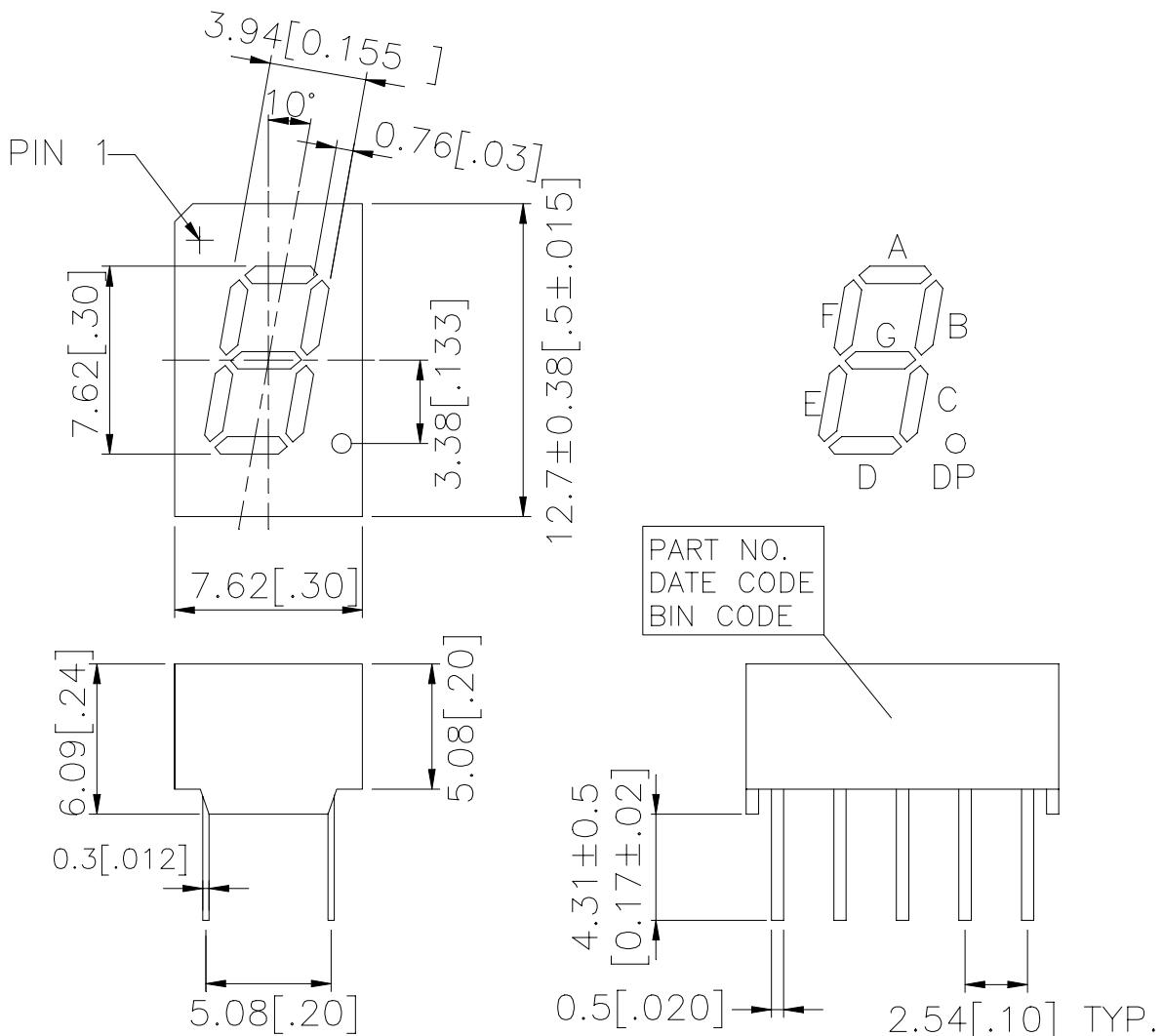
NOTES: All dimensions are in millimeters. Tolerances are  $\pm 0.25\text{mm}$  (0.01") unless otherwise noted.
