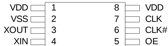
Figure 1. Pin Diagram – 8-Pin TSSOP
