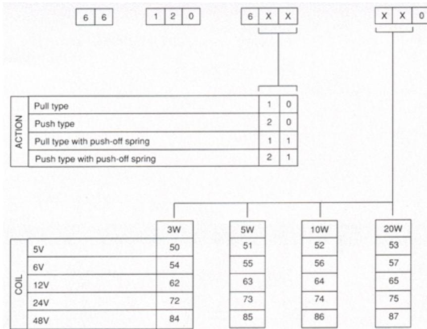
Coil Resistance, Calculate  $R = \frac{V^2}{W}$
