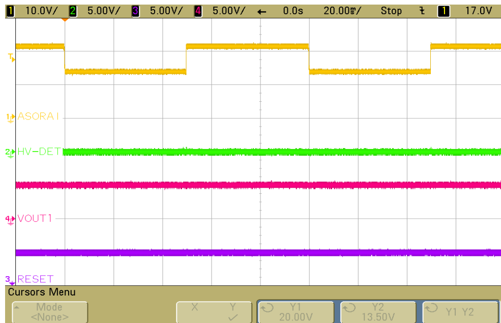
Figure 31. HV-DET Response to High Voltage – VBAT-MON Left Open
