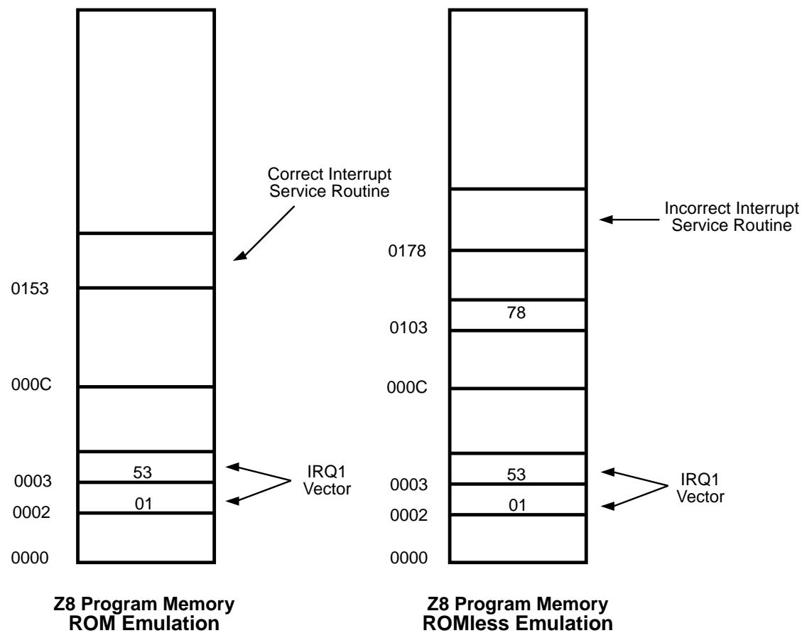
**Note:** The Incorrect Vectored Interrupt emulation only applies to the emulator. The Z89168/C68 device does not exhibit this problem.
