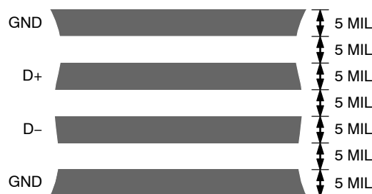
Figure 23. Typical Arrangement of Signal Tracks
