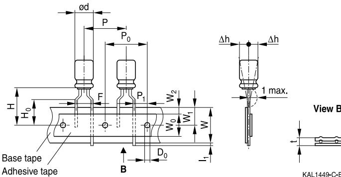
**Lead spacing 5.0 mm ( $\emptyset d = 10 \dots 12.5$  mm)**
