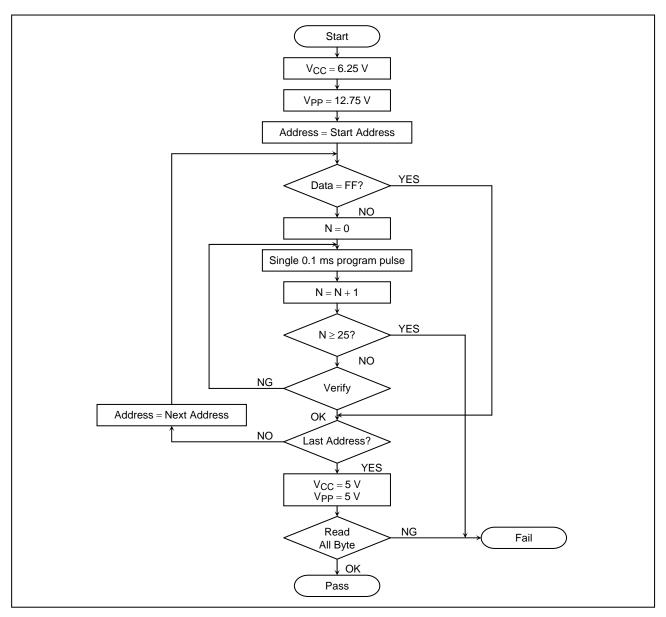
Figure 1.3.1 Flow Chart of High-speed Programming
