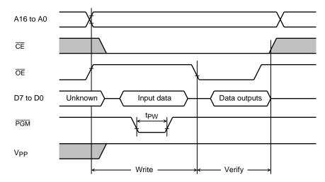
Note 1: When Vcc power supply is turned on or after, Vpp must be increased.
