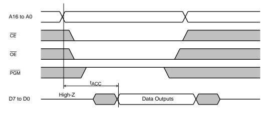
(2) High-speed programming operation (Topr =  $25 \pm 5$  °C,  $V_{DD}$  =  $6.25 \pm 0.25$  V)
