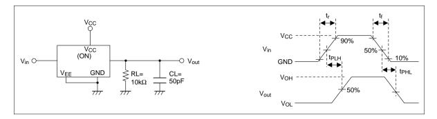
$\mathbf{t}_{\text{PLH}}, \mathbf{t}_{\text{PHL}}$ : **Propagation Delay Time** (Control Input to Switch Output)
