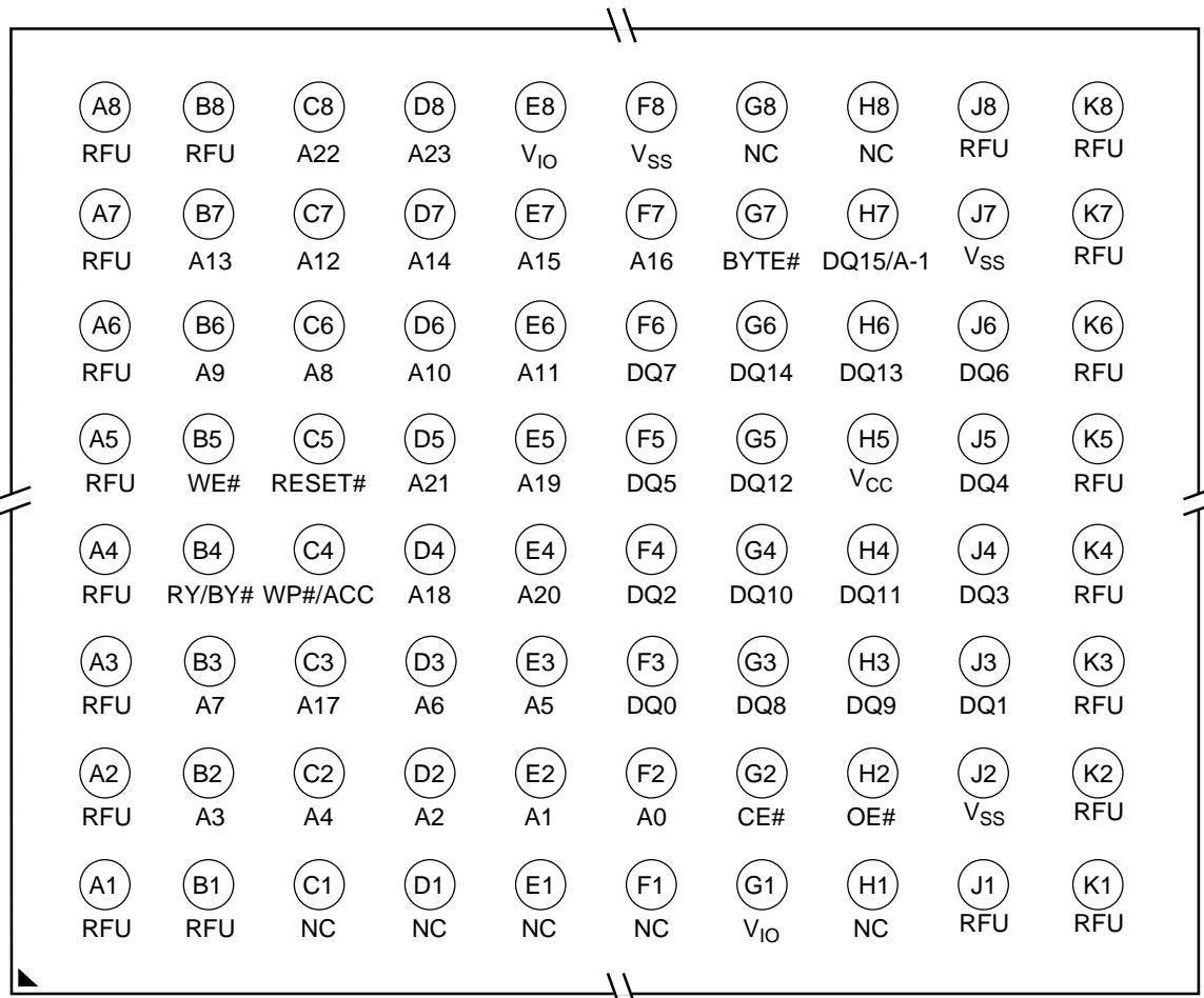
**Note:** The FBGA package pinout configuration shown is preliminary. The ball count and package physical dimensions have not yet been determined. Contact AMD for further information. RFU = Reserved for Future Use.
