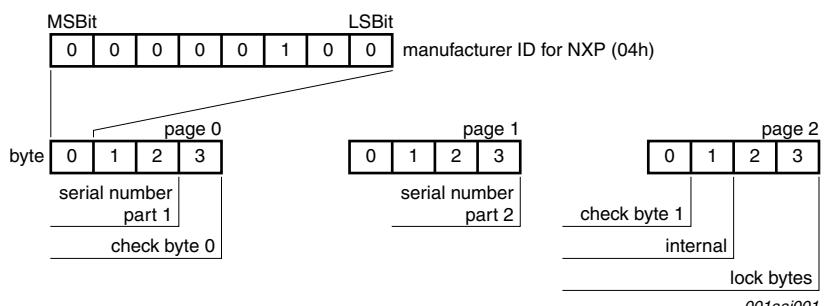
**Fig 4. UID/serial number**
