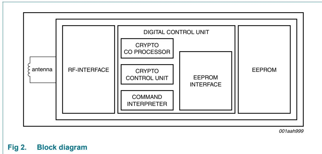
Fig 2. Block diagram
