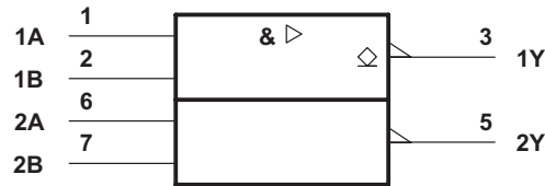
Figure 11. SNx5452B Logic Symbol
