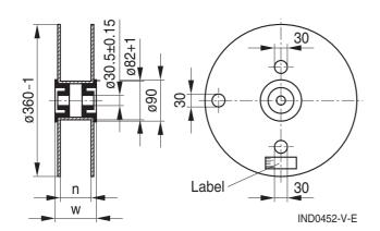
n (mm): Axial 72 +1, radial 42 +1 w (mm): Axial 84 max., radial 54 max.
