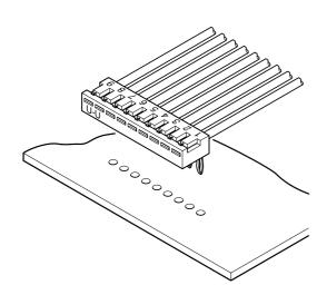
Side entry type board-in connector, with a mounting height of only 2.8mm and a thickness of 4.9mm.
