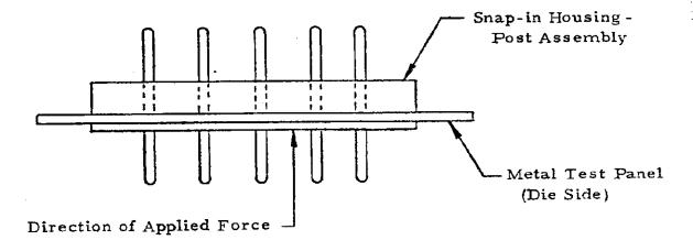
Notes: 1. Nylon housing shall be inserted into punched side of the metal test panel.
