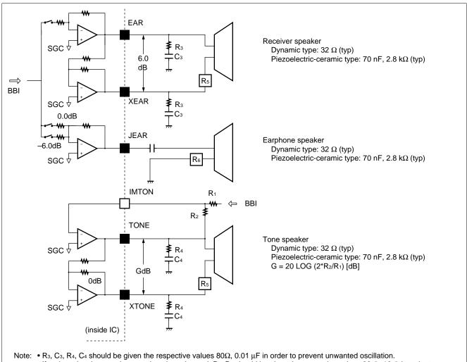
• If a piezoelectric-ceramic type microphone is used,  $R_5$ ,  $R_6$  should be given the respective values 20  $\Omega$ , 10  $\Omega$  in order to prevent unwanted oscillation.
