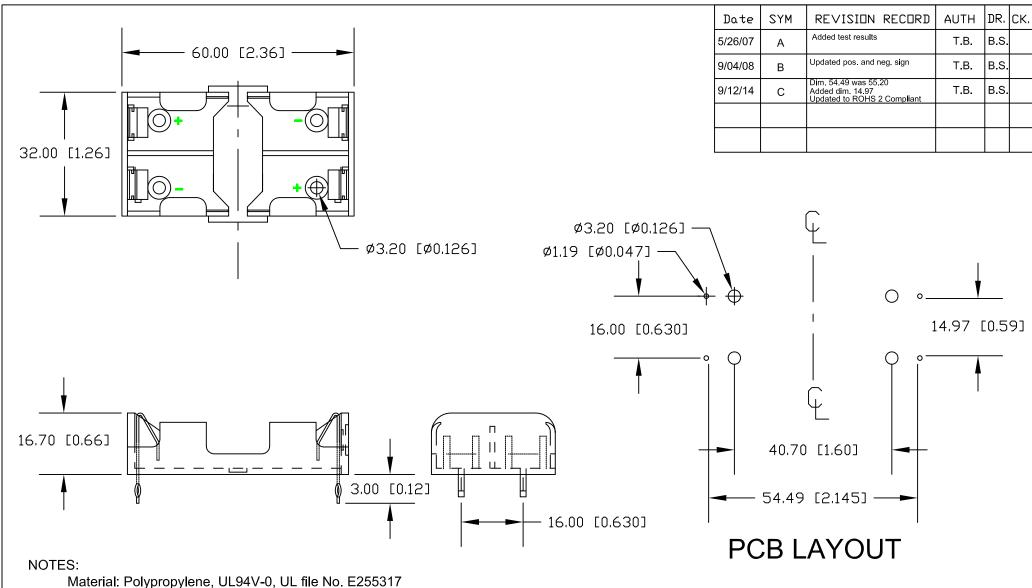
Material: Polypropylene, UL94V-0, UL file No. E255317 Contacts: 302 Stainless Steel Spring Temper, Nickel Plated
