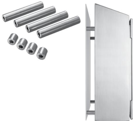
Stand-offs provide space between wall-mount enclosure and wall for better washdown accessibility. Maintains Type 4X rating. Sealing washers included. Four stand-offs per kit.
