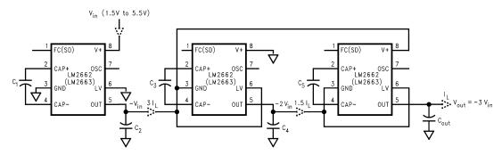
Figure 22. Generating -3V<sub>in</sub> from +V<sub>in</sub>
