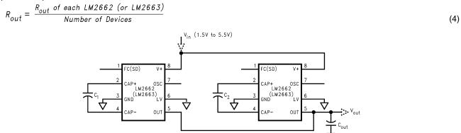
Figure 20. Lowering Output Resistance by Paralleling Devices
