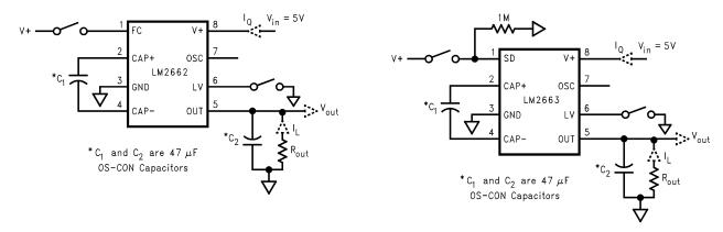
Figure 1. LM2662 and LM2663 Test Circuits
