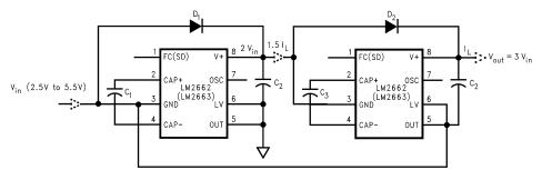
Figure 23. Generating +3V<sub>in</sub> from +V<sub>in</sub>
