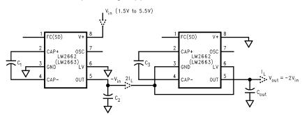
Figure 21. Increasing Output Voltage by Cascading Devices
