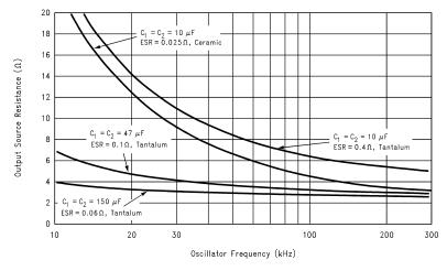
Figure 19. Output Source Resistance vs Oscillator Frequency
