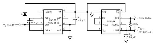
Figure 25. Generating +5V from +3.3V Input Voltage
