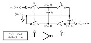
Figure 18. Voltage Inverting Principle
