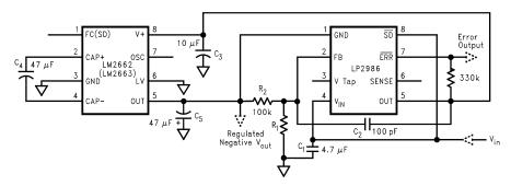
Figure 24. Combining LM2662/LM2663 with LP2986 to Make a Negative Adjustable Regulator
