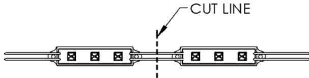
Modules can be secured onto a mounting surface with two #6 screws. Modules are waterproof and can be used outdoors. The installer is responsible for waterproofing the connection to the power source. The installer is also responsible for the use of an exterior approved power source.
