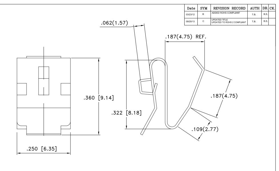
MATERIAL: 0.010" SPRING TEMPER STAINLESS STEEL, NICKEL PLATED ROHS 2 COMPLIANT
