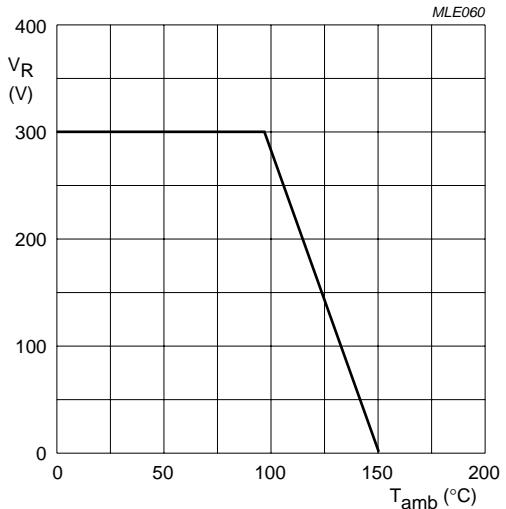
Fig.7 Maximum permissible continuous reverse voltage as a function of ambient temperature.
