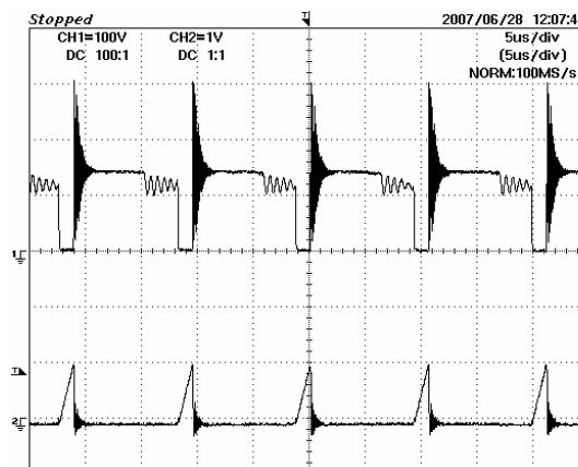
Figure 15 – 90 VAC, V_{out} = 2.3 V, I_o = 3 A Upper: V_{DRAIN} , 100 V Lower: I_{DRAIN} , 1.0 A / div, 5 \mu s / div.
