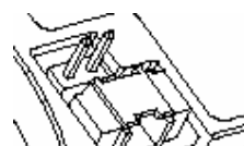
Figure 9: Master Setting for Vertical iDiskOnChip 40-Pin Connector
