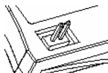
Figure 8: Master Setting for Vertical iDiskOnChip 44-Pin Connector
