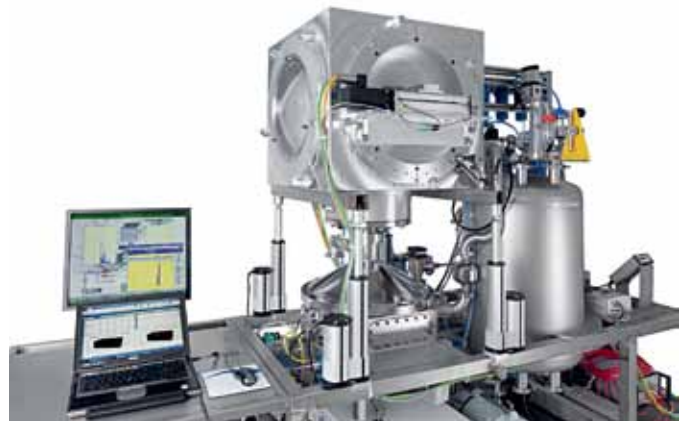
VAT particle test stand for particles > 10 nm
