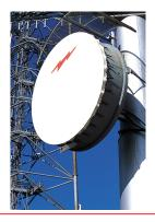
1.2 m | 4 ft High Performance Parabolic Shielded Antenna, dual-polarized, 7.125–8.500 GHz, PDR84, gray antenna, enhanced white radome without flash, standard pack—one-piece reflector
